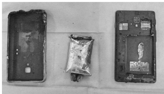
Fig. 1 - Mobile phone appearance after battery explosion. The phone was in the trouser pocket, in stand-by mode and not charging.
